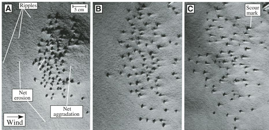
**Figure 2. Wind tunnel experiment (conducted by J.R. Steidtmann) illustrating “repulsion” and upwind migration of pebble-sized clasts on wind-erodible sandy substrate. A: Early times of 2 h experiment. B: Intermediate times of 2 h experiment. C: Late times of 2 h experiment.**
